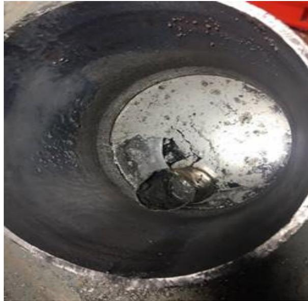
***Figure 13: Liquid mercury found in equipment***
